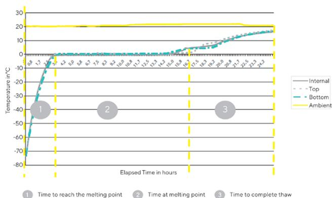
Figure 2: Celsius® FFT 2L typical thawing temperature profile
