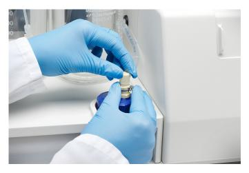
Figure 12-5: Removing Waste Tube Connector
