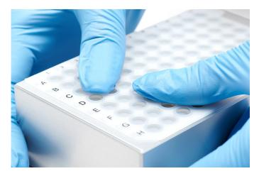
Figure 3-10: Installing Septa
