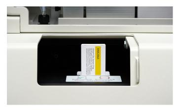
Figure 3-4: Sensor Chip Installation Port
