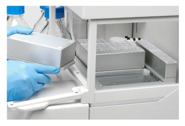
Figure 3-9: Installation of Sample Rack
