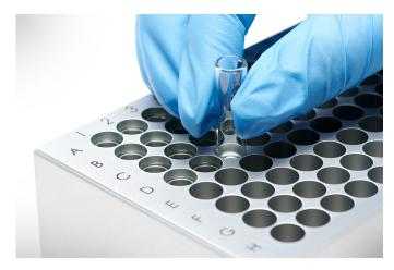
Figure 3-8: Correct Vial Orientation
