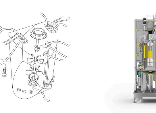
Graphical representation of the geometry of Biostat STR<sup>®</sup> Flexsafe bag; H/D = 1.8; h1/D = 1.2; d2/D = 0.38
