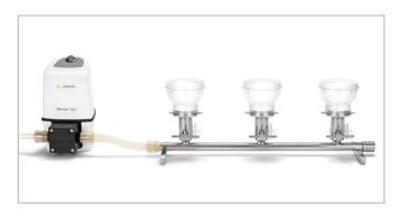
${\sf Microsart}^{\circ}$  Manifold with 100ml  ${\sf Microsart}^{\circ}$  Funnels and  ${\sf Microsart}^{\circ}$  e.jet Pump (Pump and Funnels are not included in the delivery content)
