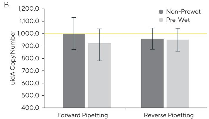
Figure 3: (A) %Error of Cq (cycle of quantification) for Pre-wet and Non-prewetting of pipette tips when pipetting Master mix. %Systemic error of Cq (cycle of quantification) and %Random error of Cq are shown. For each data point, n = 8. (B) Quantified *E. coli uidA* copy number. Yellow line indicates actual target amount. Non-prewet with forward pipetting gives the lower systemic error compared to pre-wetting. Standard Tip—Sartorius Safetyspace Filter Tips.
