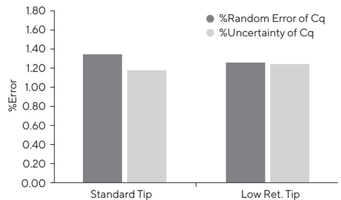
Figure 4: Percent Error for standard tips and low retention tips for pipetting of Master mix. %Random error of Cq and %Uncertainty of Cq (%Random error and %Systemic error) are shown. Forward pipetting technique was used. For each data point, n = 8. %Uncertainty for low retention tips is lower compared to standard tips. Standard Tip—Sartorius Safetyspace Filter Tips, Low Ret. Tip—Sartorius Safetyspace Low Retention Tips.
