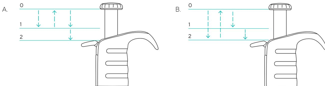
Figure 1: (A) Forward pipetting sequence and (B) Reverse pipetting sequence. For more information on these two pipetting techniques: <https://www.youtube.com/watch?v=oH-5hwC8q0>, <https://www.youtube.com/watch?v=6ZvIVNTu7Xk>
