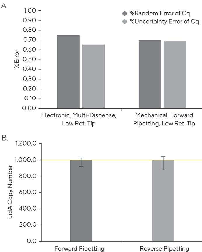
Figure 5: (A) %Error for pipetting of Master mix with electronic or mechanical pipette. %Random error of  $Cq$  and %Uncertainty of  $Cq$  (%Random error and %Systemic error) are shown. Forward pipetting was used for mechanical pipette and multi-dispensing mode for Electronic pipette. (B) Quantified *E. coli uidA* copy number. Yellow line indicates actual target amount. For each data point,  $n = 8$ . Low Ret. Tip—Sartorius Safetyspace Low Retention Filter Tips.
