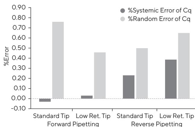
Figure 2: %Error of Cq (cycle of quantification) for forward and reverse pipetting of Master mix. %Systemic error of Cq (cycle of quantification) and %Random of Cq are shown. For each data point, n = 8. Forward pipetting gives a low systemic error compared to reverse pipetting (gray bars). Standard Tip—Sartorius Safetyspace Filter Tips, Low Ret. Tip—Sartorius Safetyspace Low Retention Tips.
