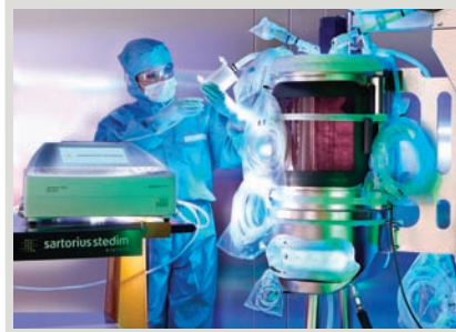
Photo 5: Sartocheck 4Plus bag tester connected to CultiBag STR 50L single-use bag (Sartorius Stedim Biotech GmbH)
