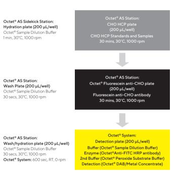
Figure 6: Flow chart of HCP assay steps on 8- and 16-channel Octet® systems with the Octet® AS Offline Immobilization Station.
