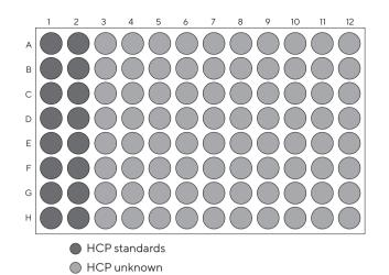
Figure 7: Sample Plate layout for incubation with biosensors on the  $\mathsf{Octet}^{\texttt{0}}$  AS Station.
