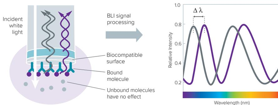
Figure 1: Relative intensity of the light reflection pattern from the two surfaces on the biosensor. Octet BLI systems measure the difference in reflected light's wavelength ( $\Delta\lambda$ ) between the two surfaces.
