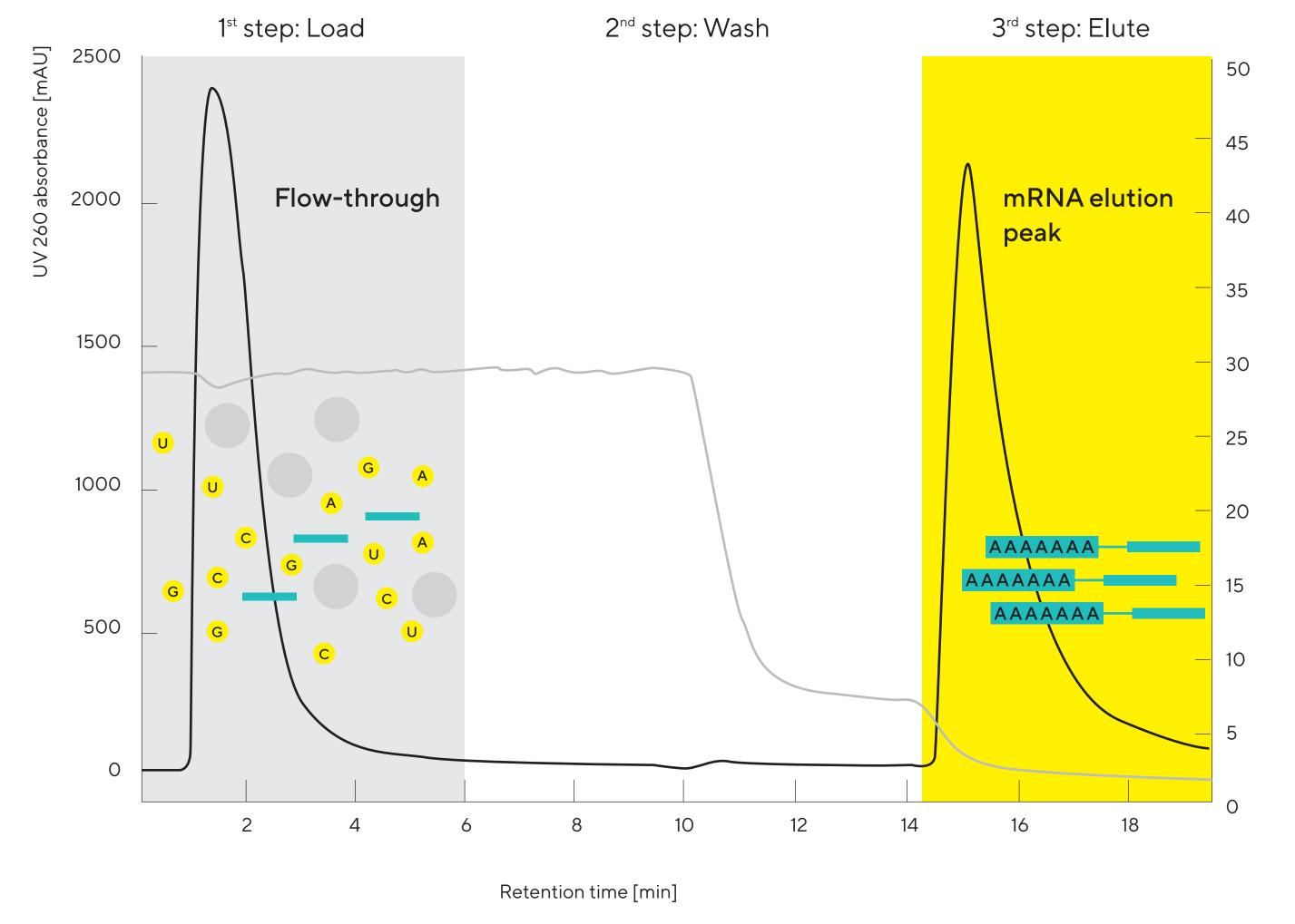
Figure 2: Chromatographic profile of IVT mix loaded to CIMmultus® Oligo dT column.
