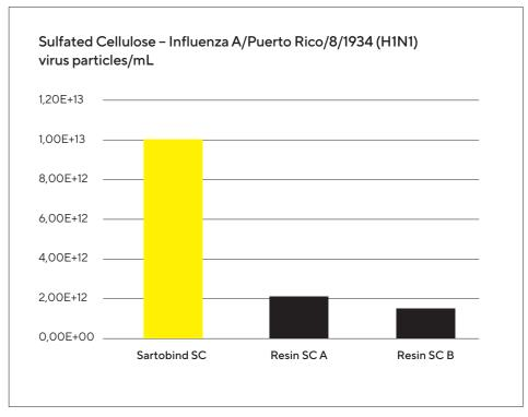
Evaluation of the recently developed SC membrane shows ~5 to 7 fold higher binding capacity of virus particles (VP)/mL, HAU/mL and ~6 fold higher flow rate than conventional resin columns.<sup>3</sup>
