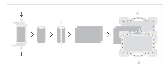
Figure 2b: Design for the cassette is derived from the capsule by cutting and creating two membrane stacks.
