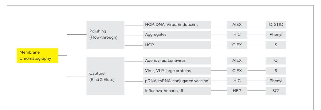
Figure 1: Typical modes of operations and applications for membrane adsorbers in the biopharmaceutical industry. Ligands: S = sulfonic acid for cation exchange (CIEX), Phenyl as hydrobhobic interaction chromatography ligand (HIC), Q = quaternary ammonium, STIC = STIC PA primary amine (salt tolerant) for anion exchange (AIEX), SC = sulfated cellulose (\*) prototype, heparine pseudo affinity (HEP)
