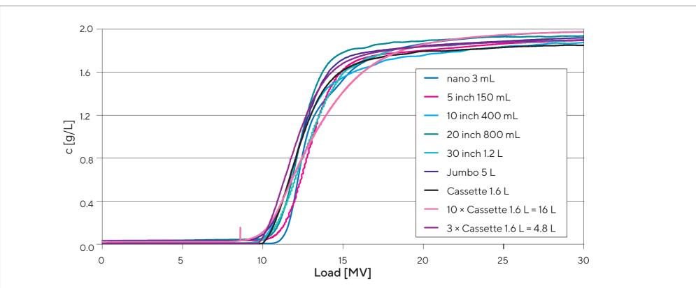
Figure 7: BSA breakthrough curves of capsules and single,  $3 \times 1.6$  L cassette and  $10 \times 1.6$  L cassette, 8 mm bed height versions.
