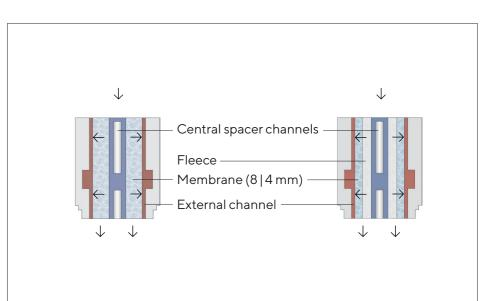
Figure 6: Design and flow path of the scalable cassette format with 8 mm (left) and 4 mm (right) bed height.
