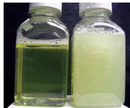
**Photo 1:** Difference in appearance between fast (LEFT) and slow (RIGHT) freezing of virus harvest fluid
