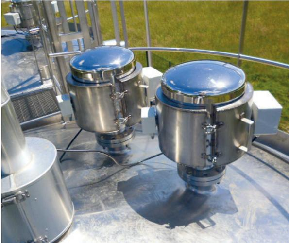
10" Jumbo Star venting filters with double jacket housing
