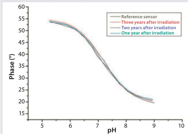
**Figure 7:** Calibration curves of used pH sensors compared to unused sensors; good comparability is achieved between a sensor exposed to 20,000 measuring cycles and an unused sensor.
