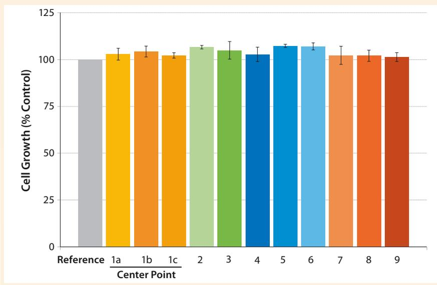
**Figure 6:** Cell-growth behavior of  $\gamma$ -irradiated bags stored under accelerated aging conditions (36-month representing 337 days at 40 °C); optimized film formulation (S80) showed excellent growth right after  $\gamma$  irradiation until the end of the study (representing 36 months). The negative control (NC) and a bag from another vendor showed initial poor cell growth that recovered after about six months. (7)
