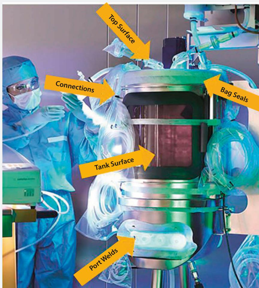
ensures reliable point-of-use leak testing of single-use bioreactor bags postinstallation and preuse in its final bag holder.
