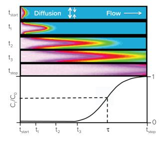
Figure 1: OneStep gradient formation in the Pioneer capillary line (top) and analyte concentration measured at the SPR flow cell (bottom). Blue indicates buffer and pink indicates sample. The gradient formation and its relationship to analyte concentration at the flow cell is illustrated using five simulated snapshots ( $t_{start} - t_{stor}$ ) in injection time.
