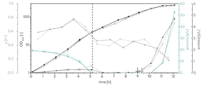
**Figure 2:** Overview of the cultivation in the Biostat® B-DCU (solid lines) with a Univessel® Glass 5 L compared to a former cultivation (dashed lines) with a Univessel® Glass 5 L. Shown is the optical density at 600 nm (black), growth rate (grey), acetate (light grey) and glucose (yellow) concentration. The start of the feed is indicated by the dashed line and the bolus feed 2 is indicated by the arrow.
