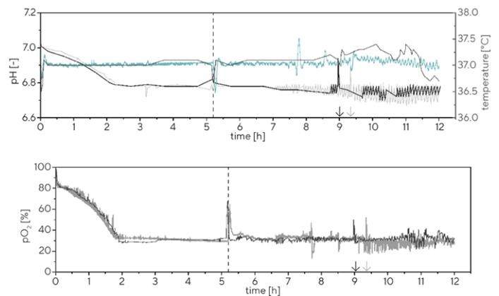
**Figure 3:** Process control of both cultivations. The  $\text{pO}_2$  was controlled by changing the tip speed and supplementing oxygen (fig. 1). Additionally, pH and temperature were also controlled. Biostat® B-DCU data were colored and data from a former cultivation were light-colored, respectively.
