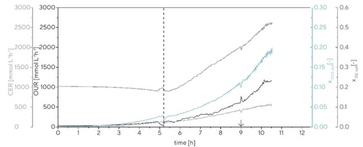
**Figure 4:** Exhaust gas measurement of the cultivation in the Biostat® B-DCU with a Univessel® Glass 5 L for oxygen (light grey) and carbon dioxide (yellow) as well calculated oxygen uptake rate (dark grey) and carbon dioxide evolution rate (grey). The start of the feed is indicated by the dashed line and the bolus feed 2 is indicated by the arrow. Exhaust gas measurement was stopped when the measuring range of O<sub>2</sub> (50%) and CO<sub>2</sub> (20%) was exceeded after 10.5 h.
