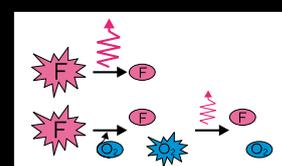
High oxygen saturation shows low emitted light intensity.
